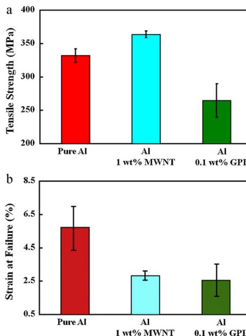
**Fig. 1.** (a) Ultimate tensile strengths of pure Al, Al-1 wt% MWNT, and Al-0.1 wt% graphene and (b) strain-to-failure.
