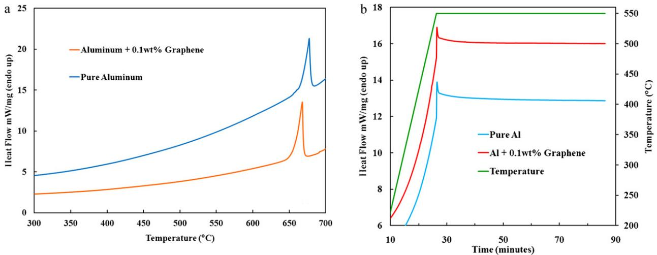
Fig. 4. Differential Scanning Calorimetry of aluminum and aluminum–graphene composites. (a) Linear heating to 700 °C, (b) isothermal hold at 550 °C.
