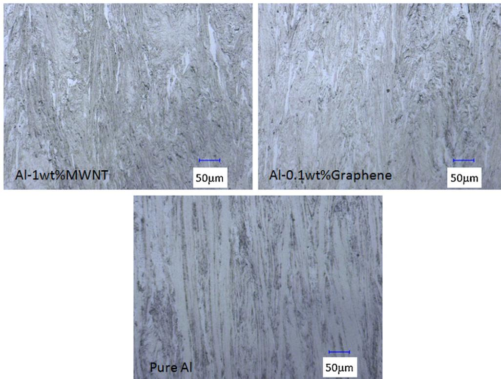
Fig. 5. Optical micrographs of extruded Al–1 wt% MWNT, Al–0.1 wt% graphene, and pure Al.
