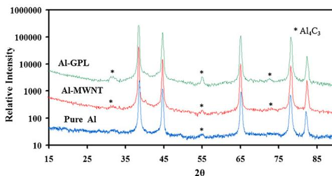
**Fig. 2.** X-ray diffraction of pure aluminum, Al-1.0 wt% MWNT composite, and Al-0.1 wt% graphene composite after extrusion.
